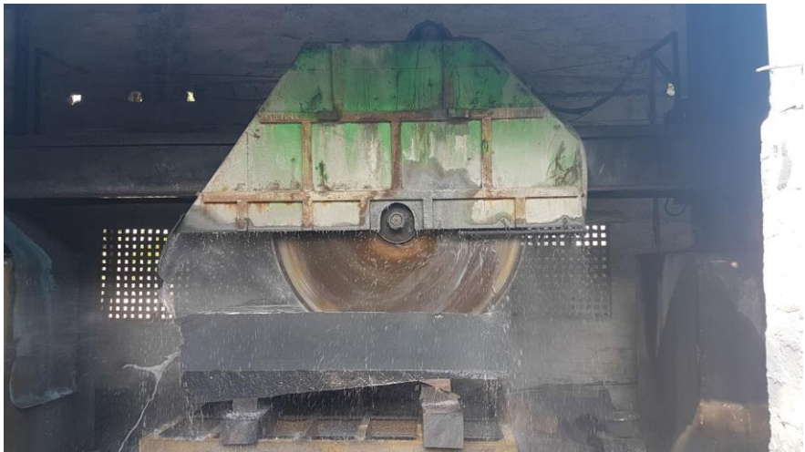
Illustration 2 – A factory that saws blocks of stone into slabs
